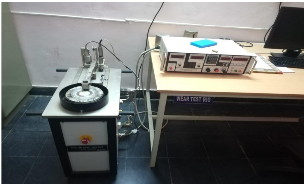
Fig 8 Pin on Disc Wear Test Machine.
