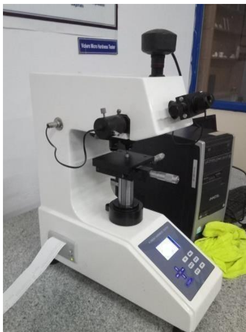
FIGURE5 VICKERS MICRO HARDNESS TESTING MACHINE
