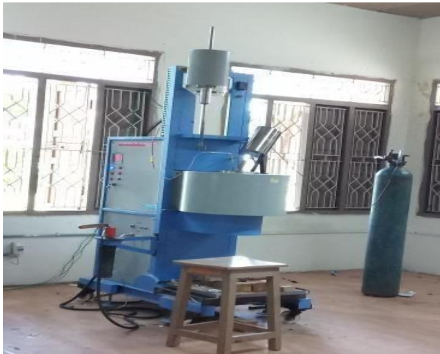
Fig 3 Bottom Type of Stir Casting.
